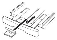
3. Insert the paper or envelopes into the paper tray. It is best to load sheets of heavy paper one at a time. If you're loading envelopes, insert them as shown. You can load up to 10 envelopes.
